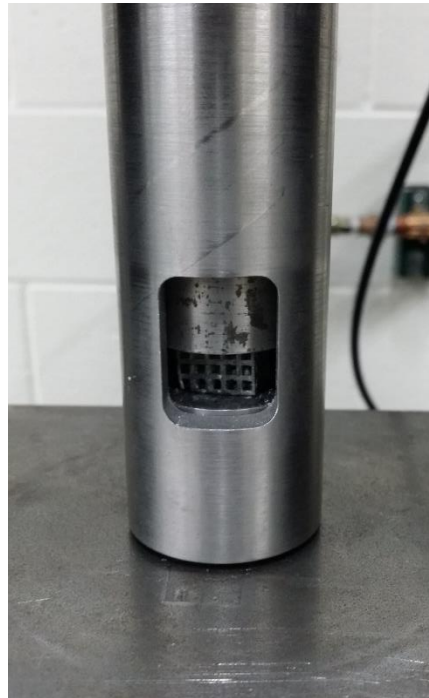
Figure 18: Scaffold in compression testing fixture
