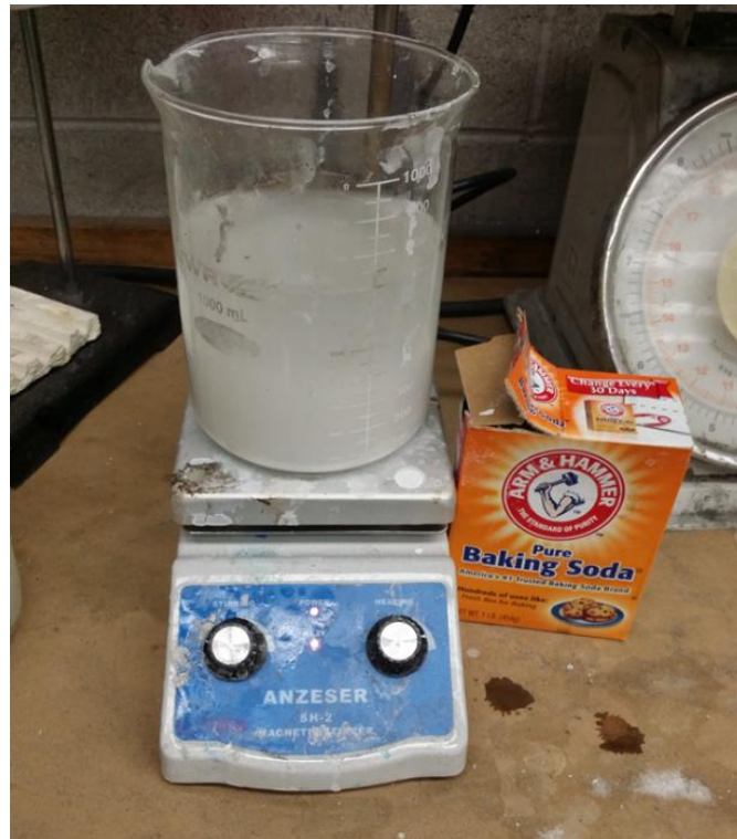
Figure 17: Apparatus of dissolving calcium sulfate from metal scaffold. Picture is a stir plate with the scaffold apparatus inside, baking soda, and water.
